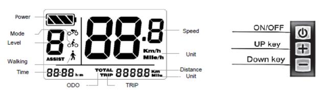
**ON/OFF** - Long press On/Off to start display. Long press On/Off again to switch off. Display off automatically after no any operation on vehicle for ten minutes (default).
